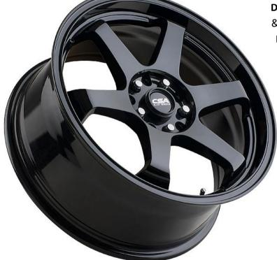
**DRIFT** has been developed with a range of 4-stud & 5-stud bolt patterns to suit many popular Small, Medium & Large Passenger, & SUV applications.
